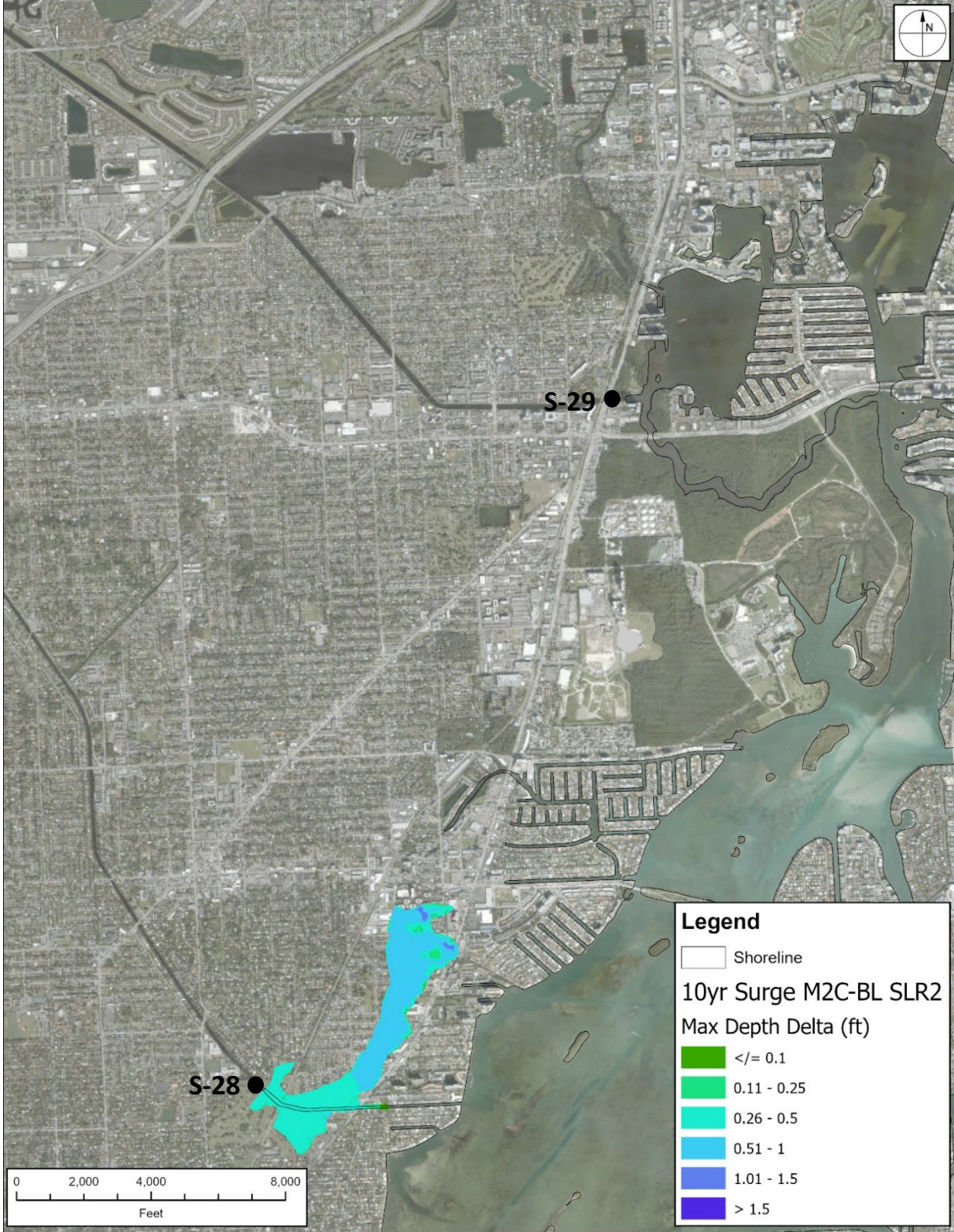
Figure 4.7 S-28 and S-29 Structures Downstream Difference in 10-yr Maximum Depths Between With and Without M2C Alternative Conditions (Sea level Rise = 2 ft)
